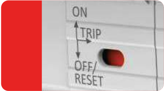
Mid-Trip Indication The knob gets in mid position while tripping because of Electrical fault.
